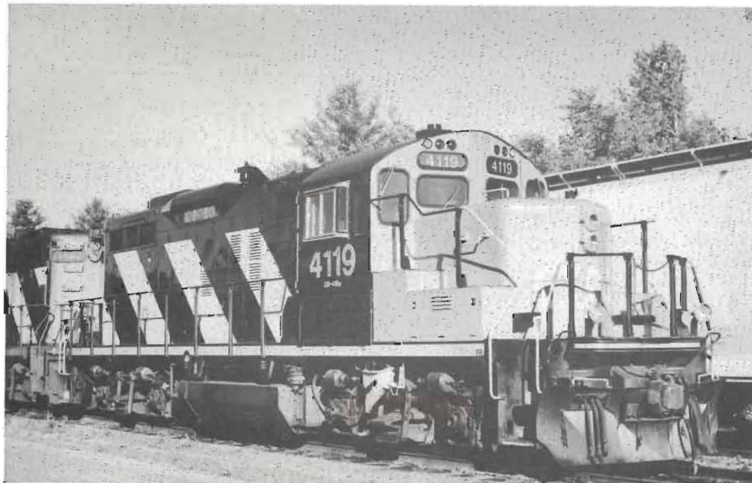
CN GP9u 4119 (ex-GP9 4211) is shown at Belleville, Ontario, in April 1990. No. 4119 is one of 66 GP9 units that have been remanufactured for continued road switcher service. Photo by David Stremes.
