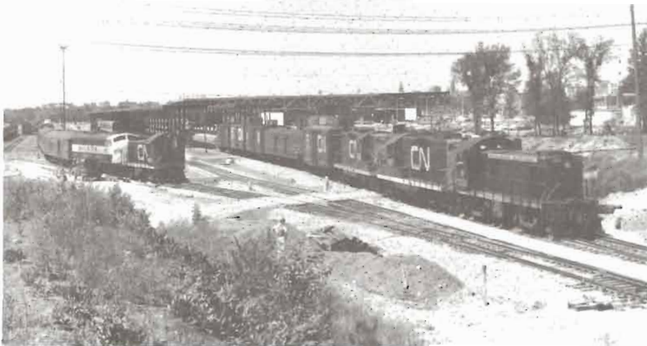
Two CN switchers were on duty the first morning of operation of the new Ottawa Union station. S-4 8059, still in its original black paint scheme, is switching train 202, an express train that ran from Winnipeg to Montreal, but also carried coach accommodation. S-4 8031 is switching out the consist of a CP Montreal train. This overall view of the station was taken at the east end throat of the yard. The foreground track served as the yard lead, paralleling the mainline east about a half mile to St. Laurent Blvd., and allowing switching to go on without interrupting the comings and goings of passenger train from tracks 1 through 4. A crossover, just off the right side of the photo, allowed access to all tracks from the switching lead. Photo: Douglas Stoltz
