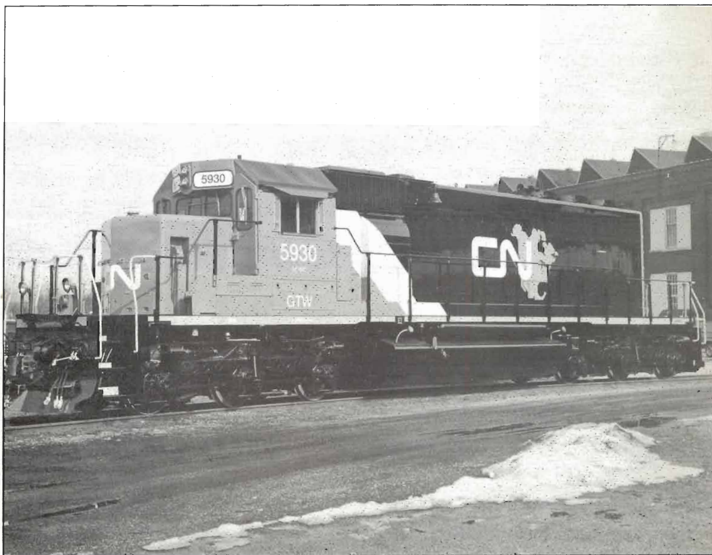
THE FIRST: CN North America SD40-2 No. 5930 (ex-Union Pacific No. 4173) is the first CN North America unit to be turned out of Grand Trunk Western's Battle Creek (Michigan) Shops in the new paint scheme. Note the small GTW under the road number on the cab. Photo by Thomas F. Bowers exposed on February 5, 1993.
