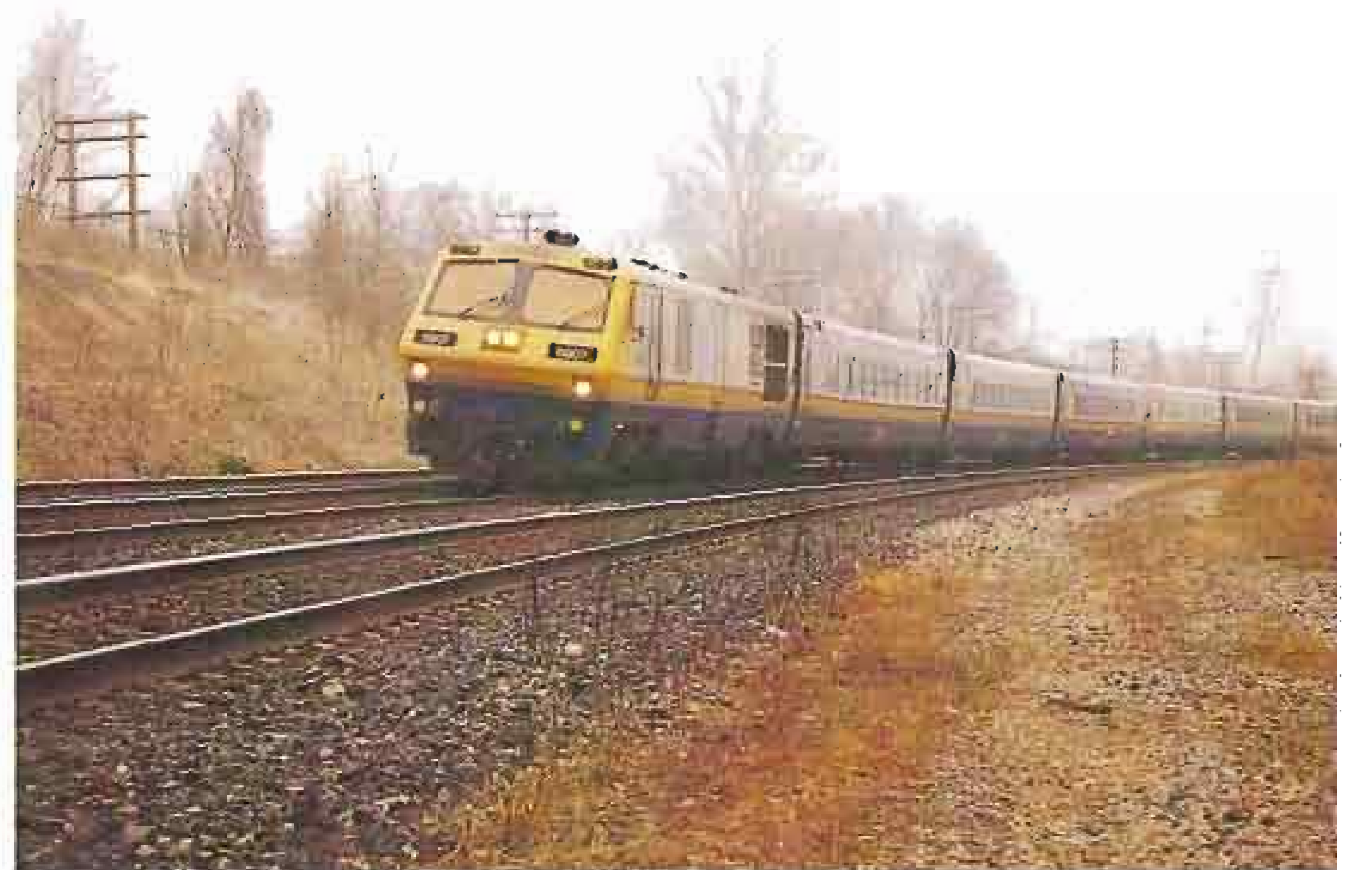
VIA LRC-2 6907 hastens Montreal-Toronto train 53 out of Guildwood, Ontario, on April 2, 1999. Note that only the first three cars have their tilting mechanisms engaged. Photo by Jason Shron.
