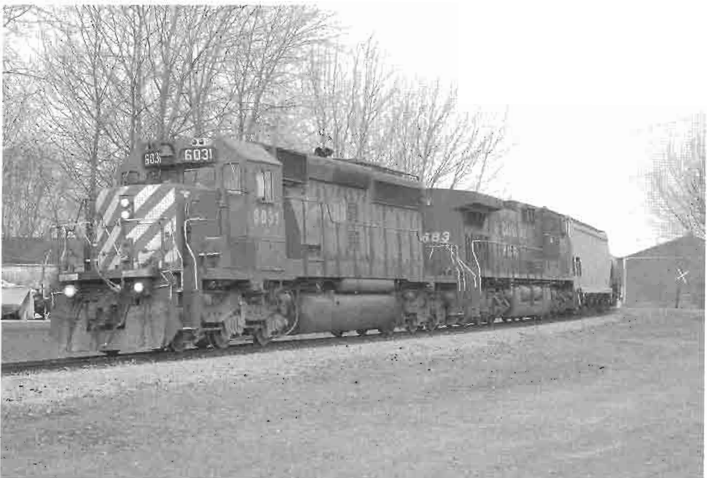
In only three days, trains through Dresden, Ontario, will be a memory, but it is business as usual as Train D725, powered by CP SD40-2 6031 and CP AC4400CW 9683, rounds the curve heading to Chatham on January 28, 2006.
