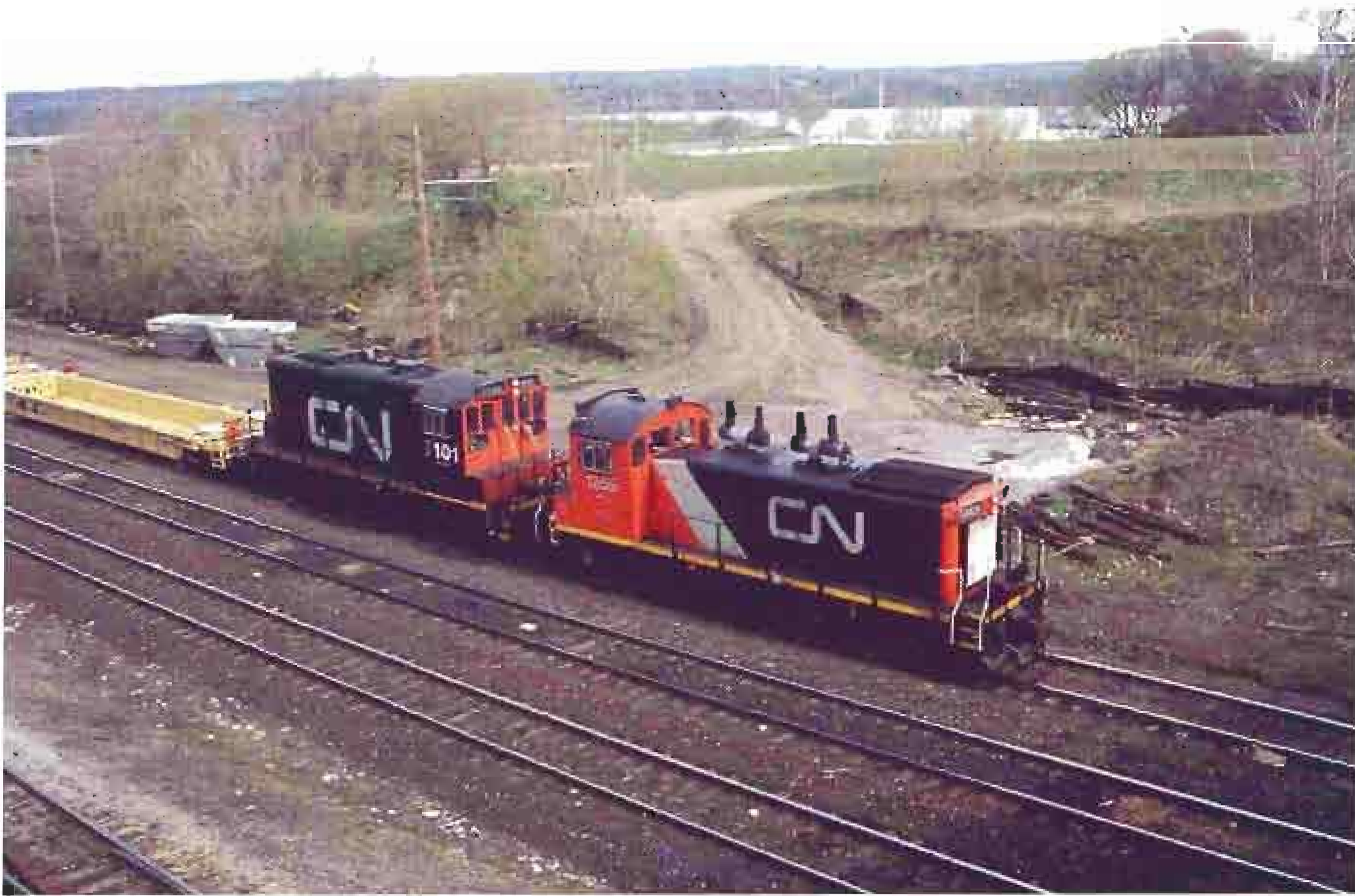
CN SW1200RS 1355 and SW1200RM 7101 switch CN's Stuart Street Yard in Hamilton, Ontario, on April 30, 1994. Photo by Jason Noe.
