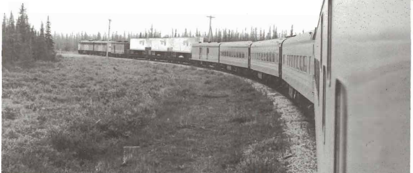
VIA Train 93 is being wyed prior to backing into the station at Churchill in July 1990. The Winnipeg-Churchill train is the only passenger train in Canada which regularly carries intermodal piggyback shipments. Special flat cars have been modified for passenger service by the addition of steam lines which pass heat from the steam generator unit behind the two FP9Au units to the trailing passenger equipment. The intermodal shipments are handled between Thompson and Churchill. Photo by Douglas N.W. Smith.
