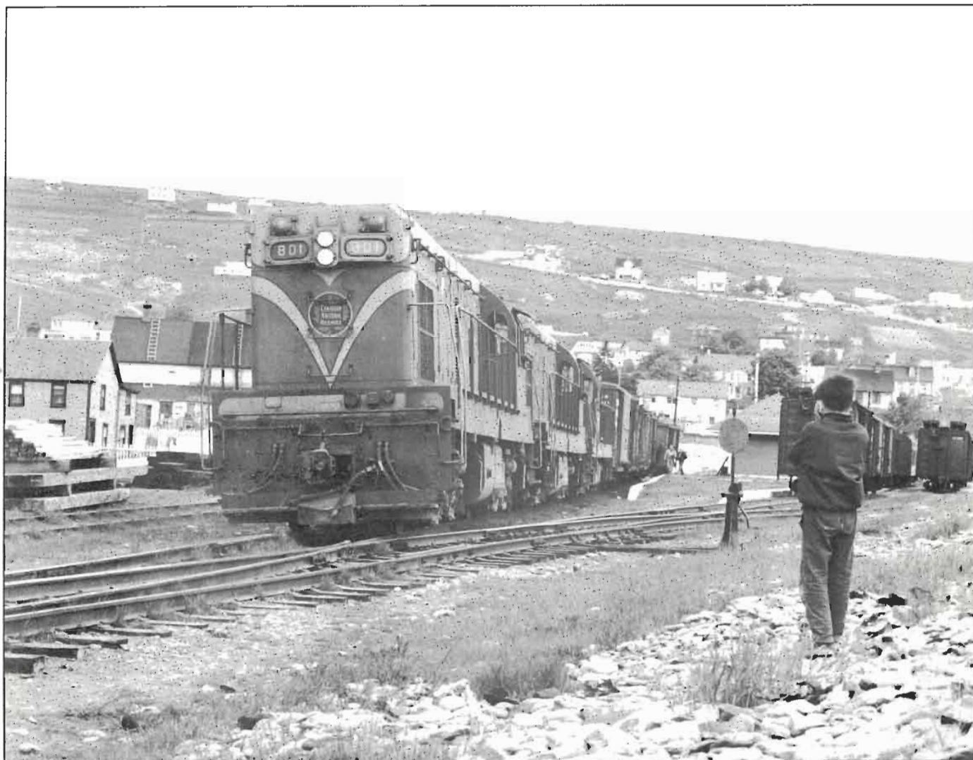
In a time-honoured pose, a small boy holds his ears in deference to the horn blasts of Canadian National Train M212, switching at Carbonear, Newfoundland, prior to its departure for St. John's on June 22, 1967. The mixed train is powered by GMD-built Model G8 No. 801 and two sisters. The 42-inch gauge tracks were abandoned in the 1980s, however, G8 No. 803 is displayed at Carbonear for future generations to see. Photo by James A. Brown.
