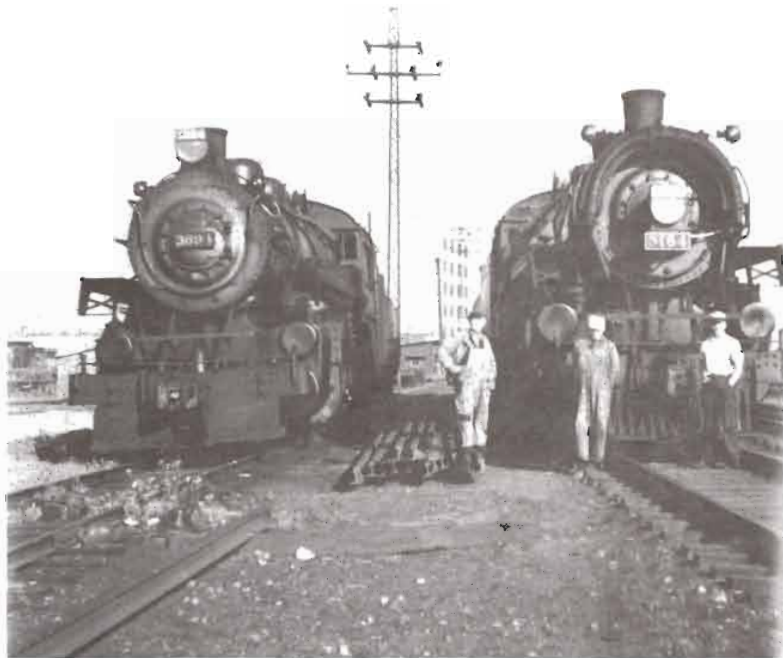
CP 2-8-2, class P1e, No. 5164. Also built by the Montreal Locomotive Works, in 1913, she'd seen lots of modifications over the years, including the odd looking Coffin Feedwater Heater/Pump system. The author was working with the engine when this photograph was taken at Hochelaga, Quebec, in 1951. Photo by the author.
