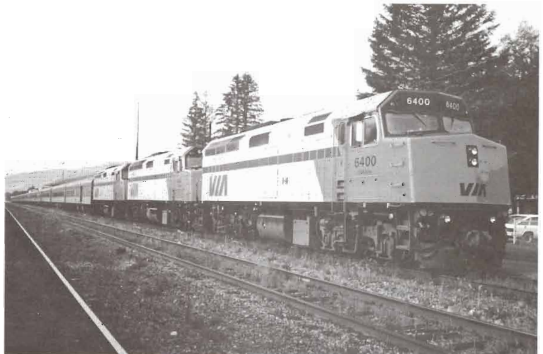
VIA F40PH-2 6400 leads two sisters and 17 cars of the "Canadian" through Blue River, B.C., on July 20, 1993. Normally the "Canadian" operates with two units. Photo by Paul Bloxham
