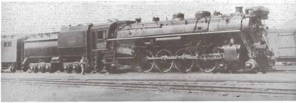
CN 6057 in the early 1930s, likely at Jasper, Alberta, before the removal of the Elesco feedwater heater. Collection of Philip Jagó.
