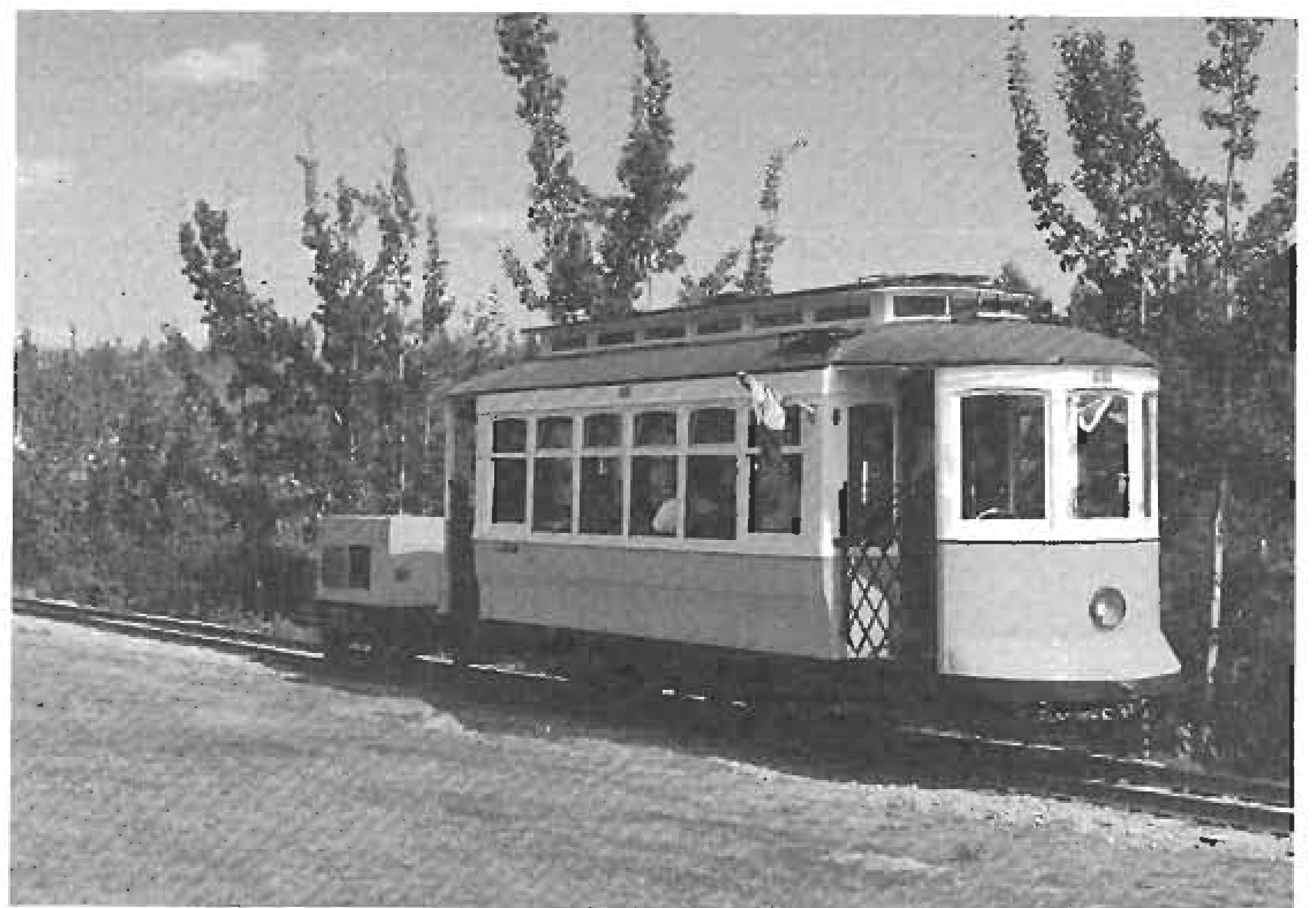
Whitehorse Waterfront Trolley 531 with attached generator for power as it travels along the original WP&YR right-of-way in August 2002.
