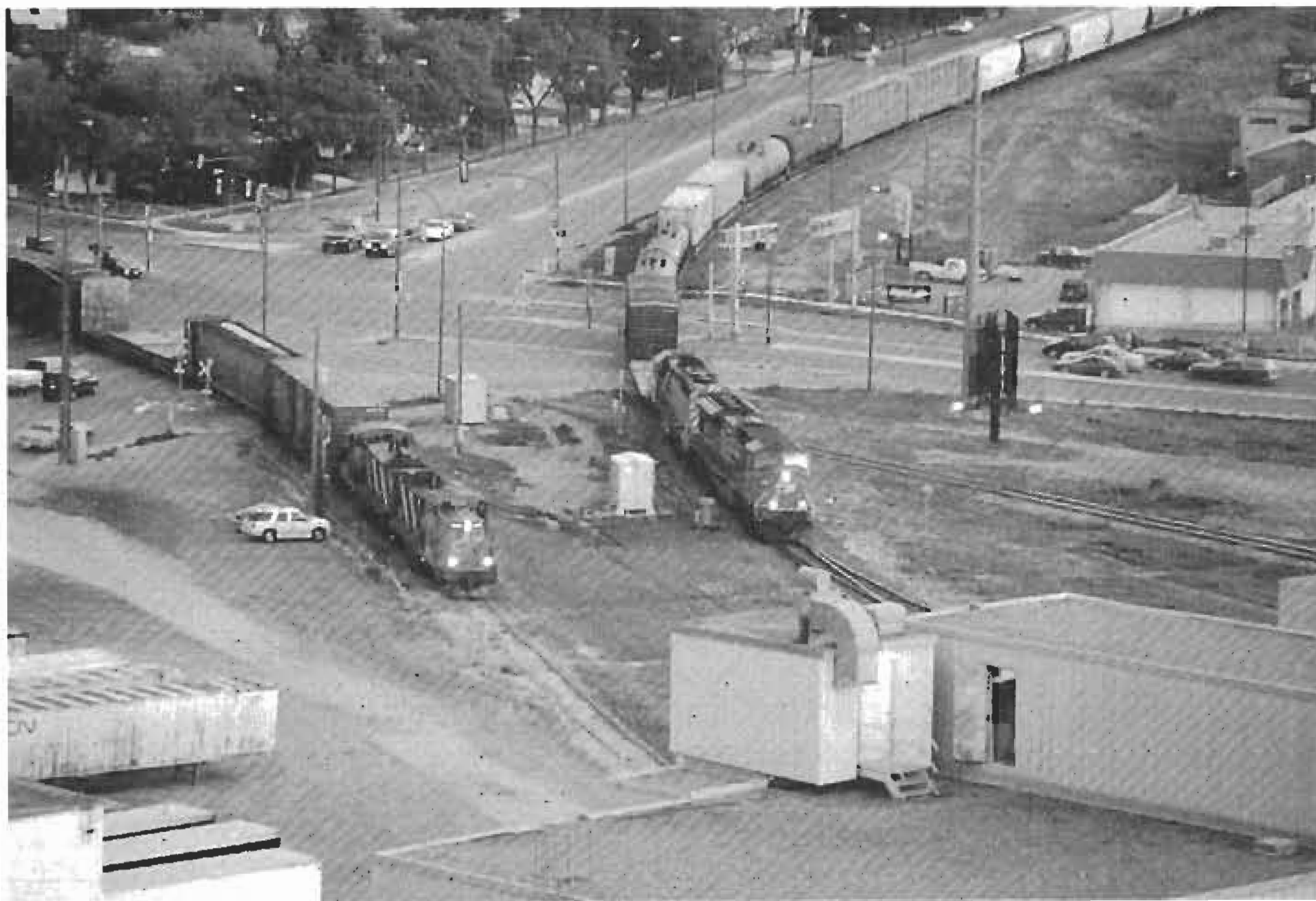
Above: Canadian Railserv lightweight RS-23 8013 (nee CP 8013) is at the Transalta Sundance plant near Wabamun, Alberta, on July 26, 2000. It is switching covered hoppers through the fly ash loading facility, the ash generated by burning coal at this power facility. The ash is interchanged with CN. Photo by Fred Clark.
