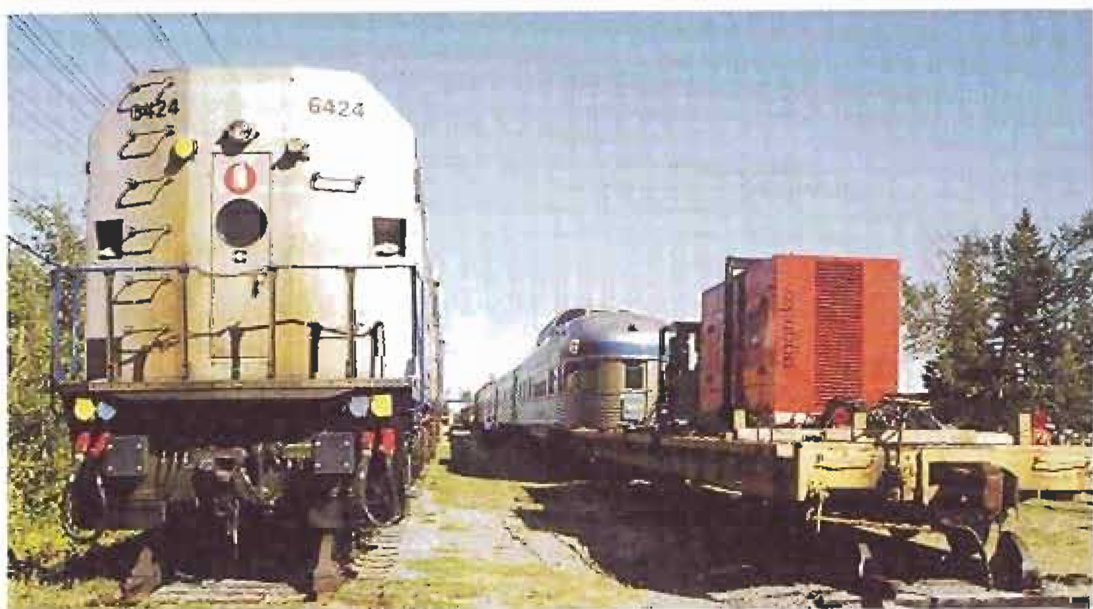
On the back track at CS&TM on September 25, 2002, was F40PH-2 6424, displaying her modified coupler to mate with the Renaissance equipment. Sisters 6425 and 6426 are similarly modified. Note the two anti-climbers. Photo by Charls Gendron.
