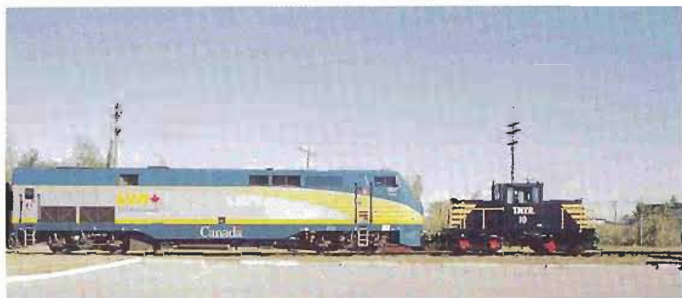
Age before beauty, and don't you look down your nose at me!! The Society's ex-Thurso & Nation Valley, General Electric, industrial switching locomotive No. 10, built by GE in 1946, stands before GE No. 907, built in 2001. Our switcher produces all of 300 HP, compared to the 4,250 of her modern sister, however, ours weighs about one third of the total of the 907 despite her diminutive size. Photo by Duncan du Fresne.
