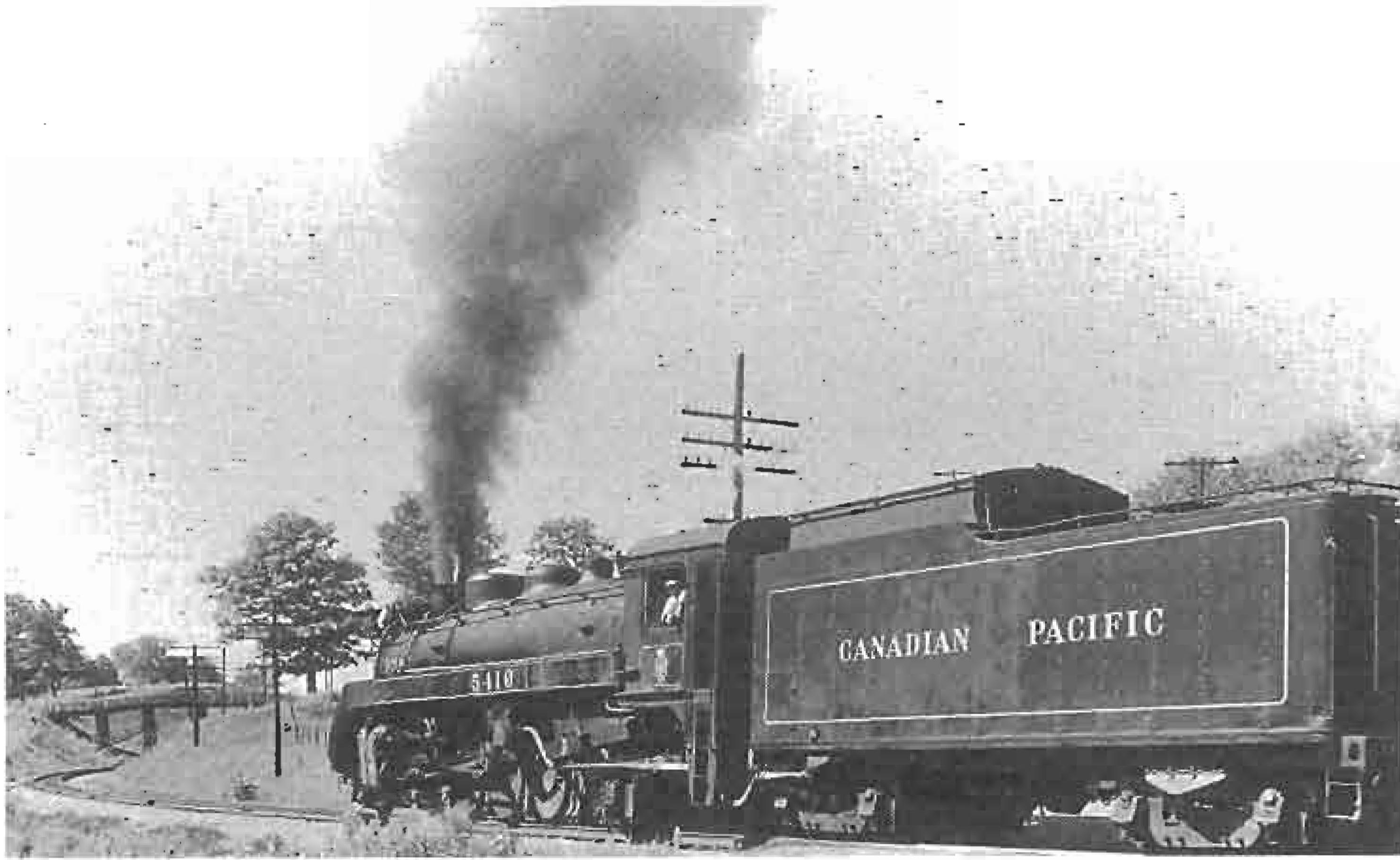
CP Mikado 5410 digs into the grade to Orrs Lake, Ontario, with a westbound freight in the late 1950s. No. 5410 was built by Montreal Locomotive Works in August 1940 and was scrapped in November 1961. Collection of Bob Layfield.
