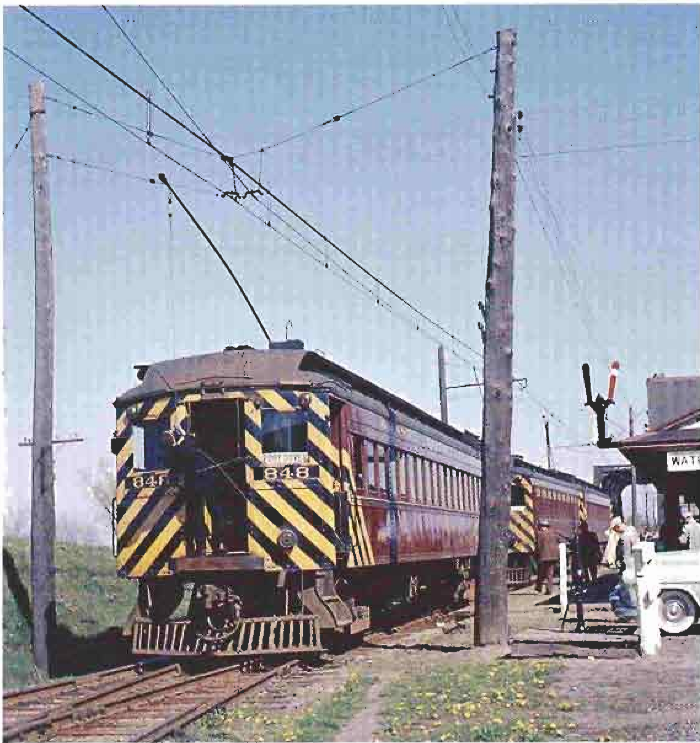
The chain across the end door was not just for restricting access. Here, it is serving very well to enable the trainman to change the trolley pole to the correct wire. With two-man crews the railway did not need trolley frogs. The train is at Waterford on May 1, 1955, waiting for the NYC train to arrive with the last run excursionists.
