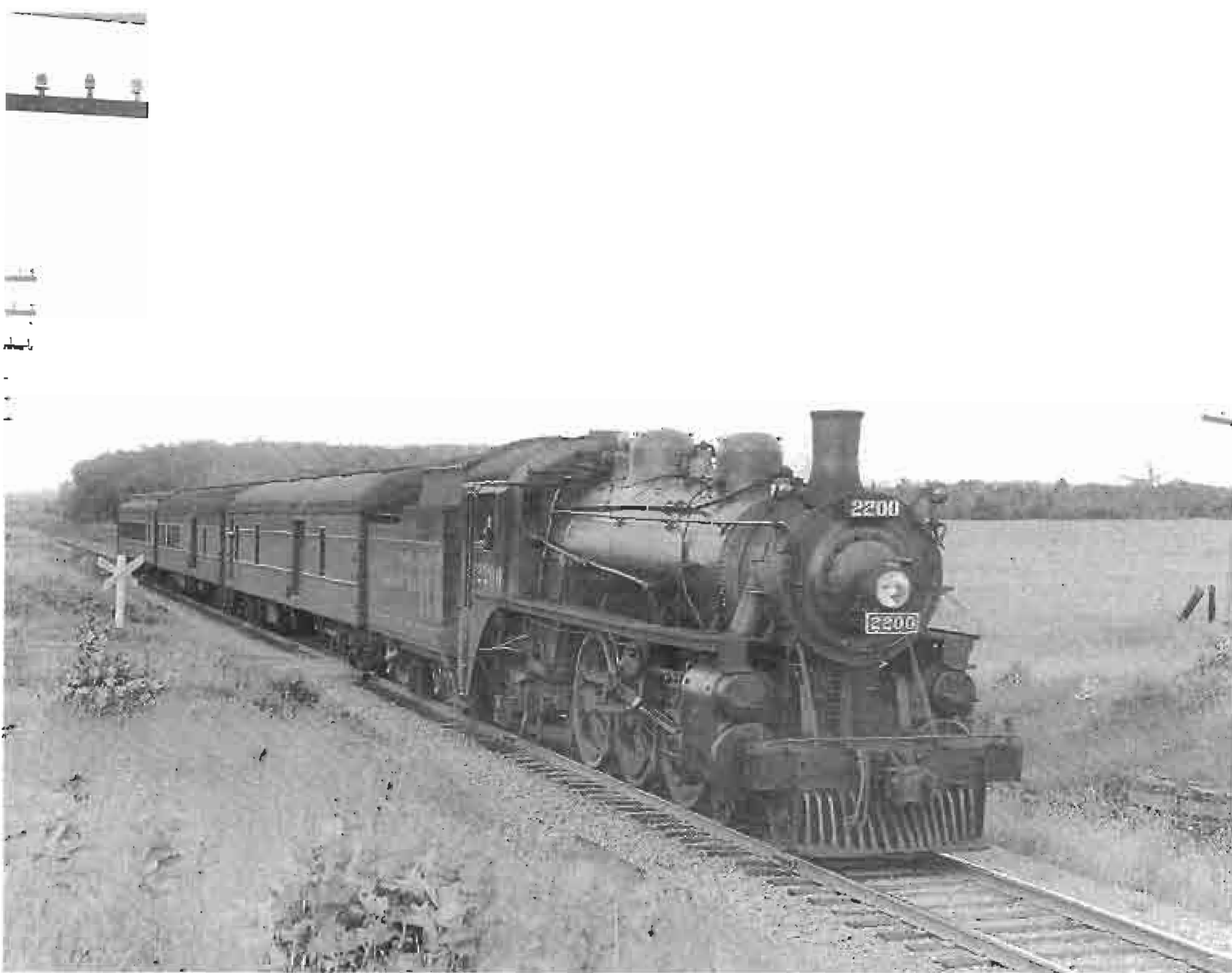
Train No. 557 is on the Carleton Place sub. near Westboro on June 27, 1956. Unlike sister 2218 (see Page 20), the 2200 is stoker equipped, has a vestibule cab, and the large 8,000 Imperial Gallon tender. Photograph courtesy of Al Paterson.
