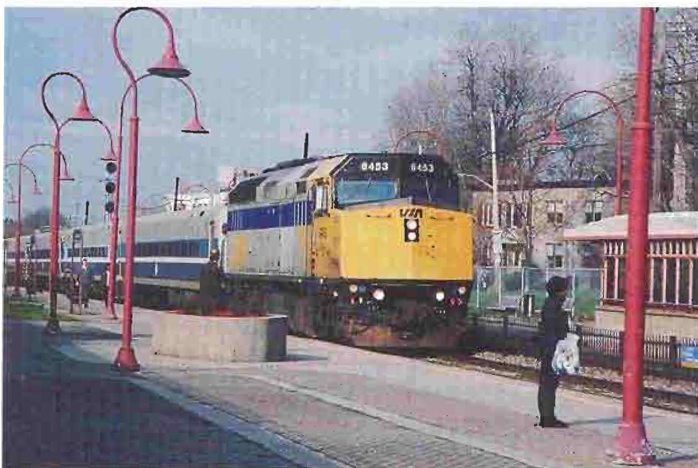
Leased VIA F40PH-2 6453 stops at Montreal West with Train #16 from Vaudreuil on May 2, 2005. The train includes 6 of the 24 Bombardier coaches built for AMT's predecessor STCUM in 1989.
