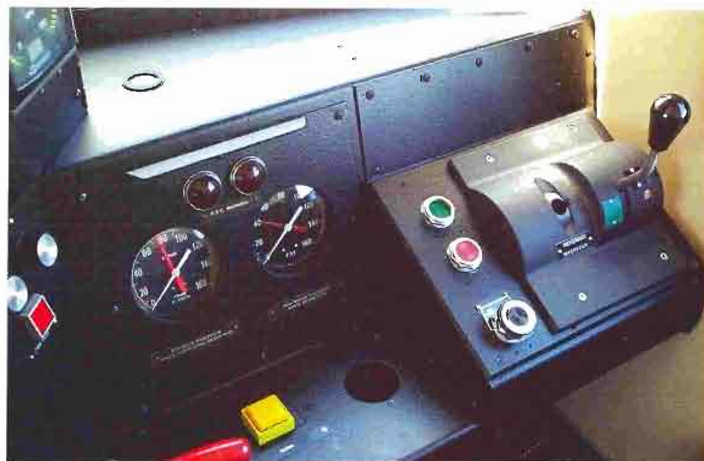
The desktop control panel in Cab Car 211 after refurbishment in 2002. Changes included a combined analog-digital style larger design speedometer, the whistle cord replaced by a button, the handheld radio moved higher up on the left side panel, plus an integrated camera.
