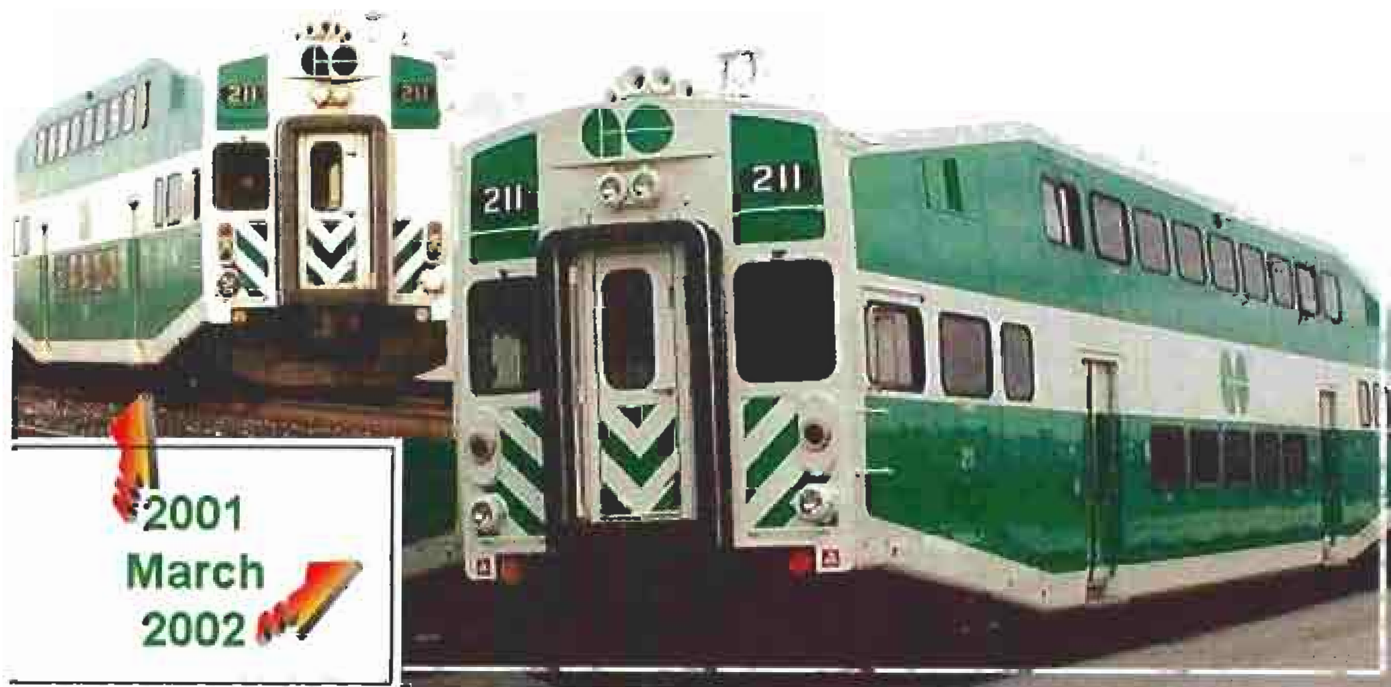
A comparison of Cab Car 211 before and after being refurbished in 2002. Note the cast bell has been replaced with an electronic bell, changed classification lights, the additional windshield, the addition of an Electrical Warning Safety Sticker, and the front hand rails have been changed from green to white.
