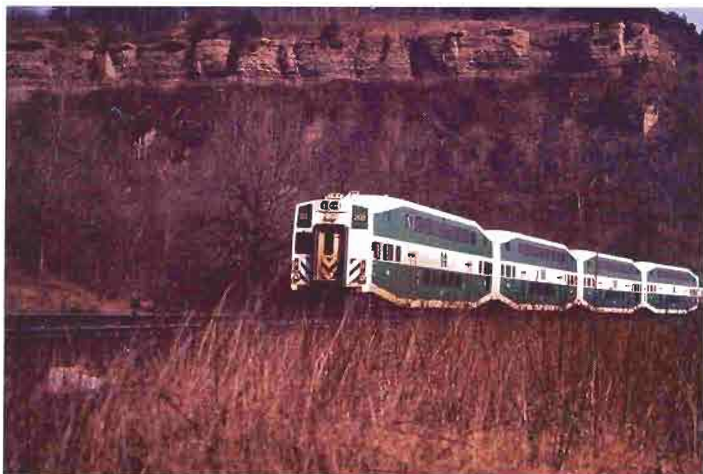
In February and March 1992, VIA experienced several broken axles on their LRC coaches. GO equipment was utilized on several Toronto-Windsor-Toronto trips. Cab Car 200 made four trips, powered by F59PH 545. Some trips were powered by a VIA unit with a GO APCU providing head-end power at 575 volts (VIA output is 480 volts).
