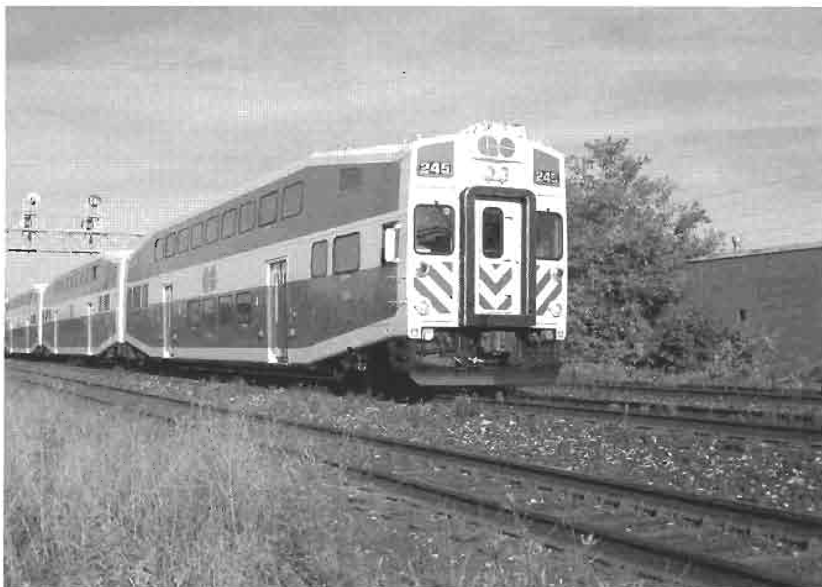
Cab Car 245, one of four delivered in 2004, sports an electronic bell, only one red classification light on each side, a mini-snowplow, two pairs of door step lights, and a full length mirror on both sides of the cab.
