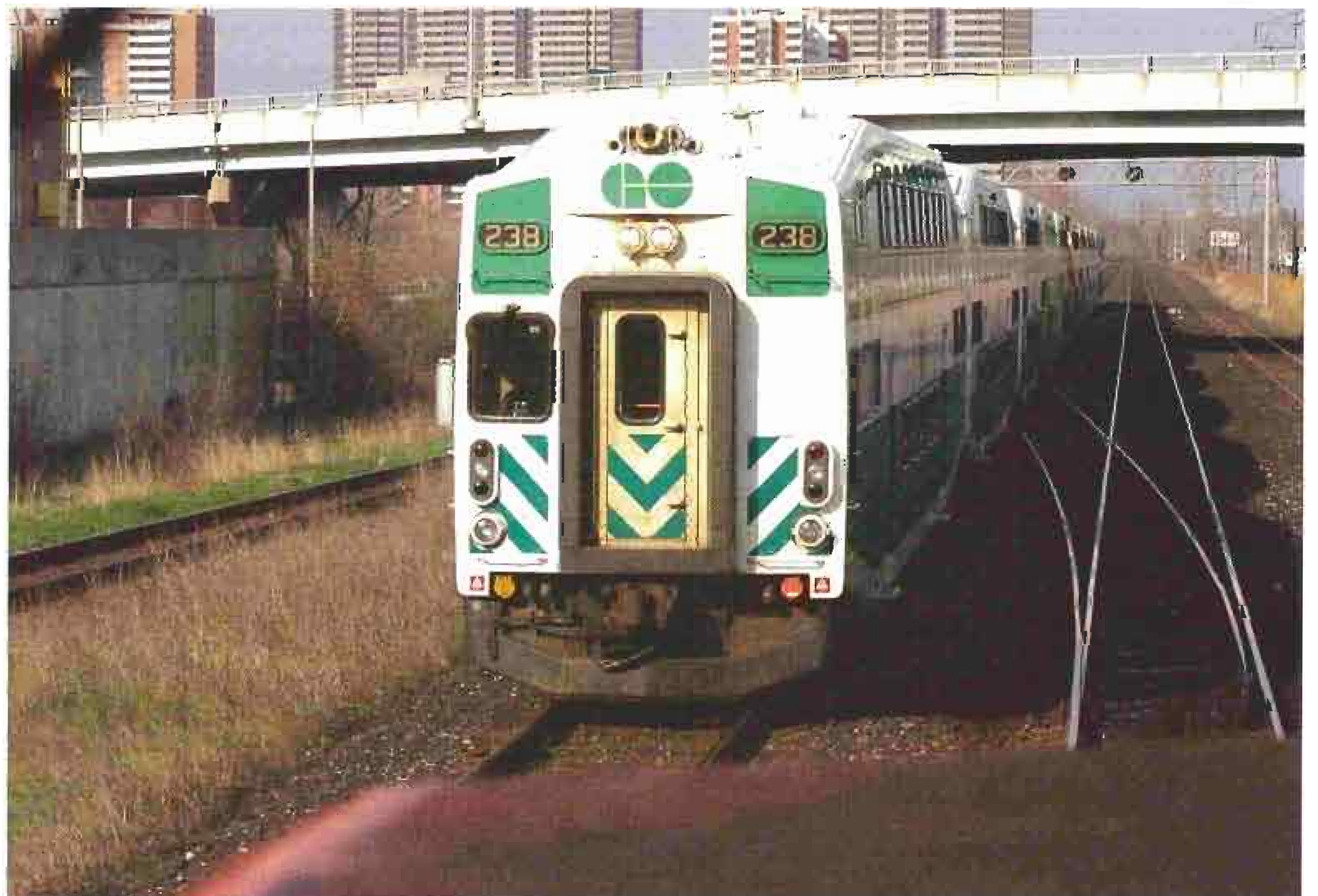
Cab Car 238, delivered in 1991, carries her original cast bell, five-chime whistle (no bug screens in the whistle) in a two-bracket whistle frame, and a full width pilot.
