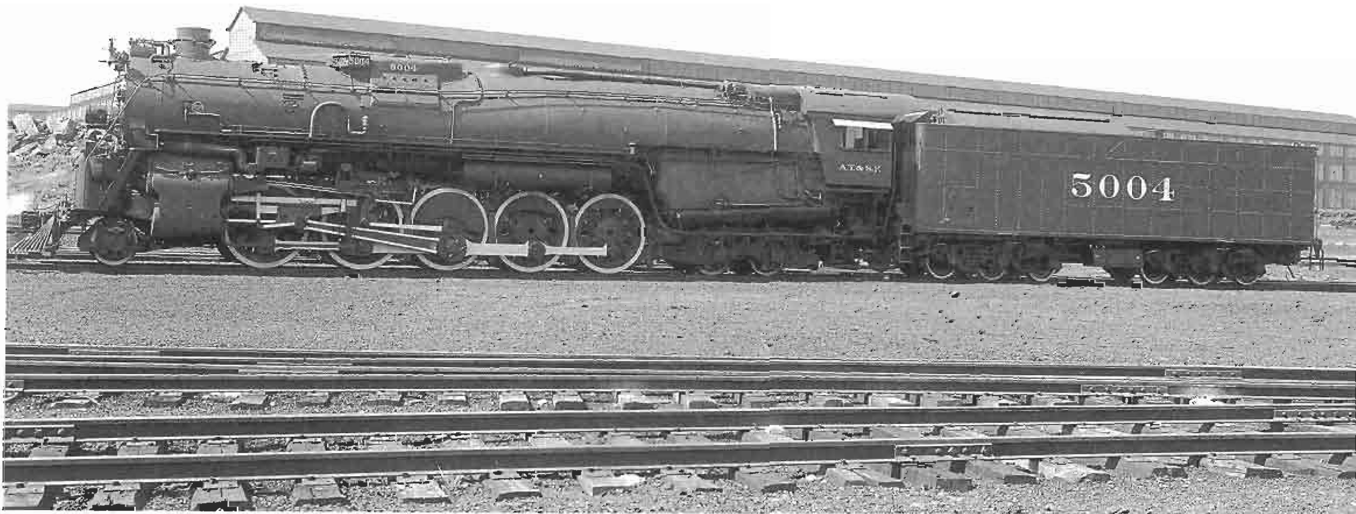
AT&SF 2-10-4 5004 with those 74" diameter drivers. That's a pretty lanky freight engine. That tender is big, but the one used on their massive 4-8-4 was even bigger. Photograph courtesy of the AT&SF RR.
