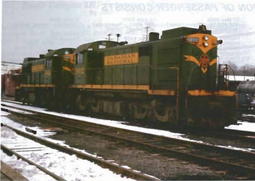
Top Left: Canadian National RSC-24s 1802 and 1803 pause at Brockville, Ontario, in March 1966. CN 1800-1803 were the only RSC-24 units built by Montreal Locomotive Works. They contained the 244 series engines removed from FPA-2 6751 and 6755 and FPB-2s 6851 and 6855 that received 251 series engines in 1958. The short hood on the RSC-24 contained the electrical cabinet - a unique feature. Photo - BRS Collection.
