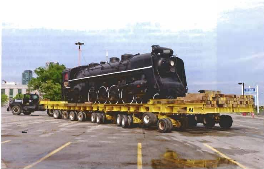
Top Left: Loaded and ready to go at 140 tons (dry weight) and with 64 wheels on the ground, 6213's float is put through its paces on a wide sweeping turn away from the CNE site of 49 years. This practice turn on June 8, 2009, the day before the actual move, was a familiarization exercise inasmuch as it was McCulloch's first experience at moving a locomotive. It was also one less turn to be done in a tightly-scheduled program. Photo by Richard McQuade.
