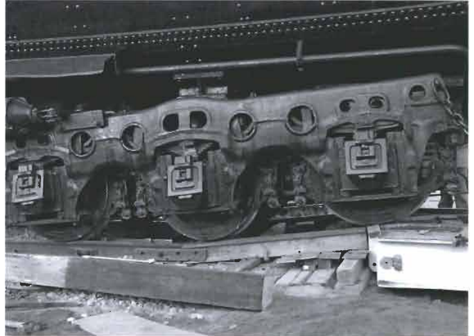
Unloading 6213's truck tender was easier said than done. Getting the first truck down a shifting prefab ramp was a nerve-wracking experience. The solution of making a temporary ramp for the second truck produced a more sure-footed alternative but the middle journal box bottoming out while the outer one's was almost flattening their springs, it seems to have tested the limits of the truck design (and taken the weight off the rails). Photo on June 4, 2009 by Richard McQuade.
