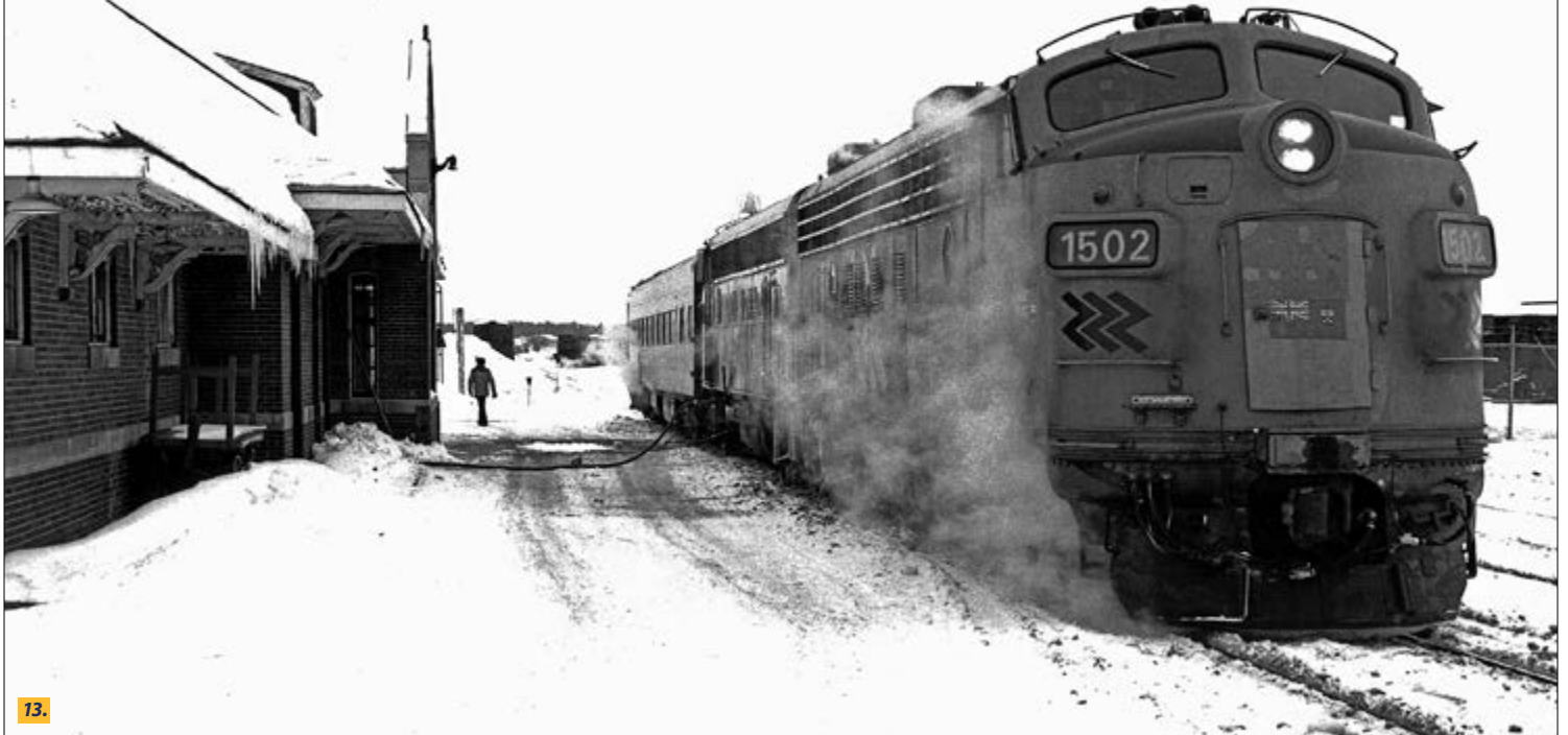
13. The Northland has just arrived at Kapuskasing. Overnight, the temperature had dropped to -34°C. By the time the train got to Kap it was up to a balmy -26°C. Though fuel was not a problem, the cold weather had caused the steam generators to use up so much water that the tanks had to be refilled before returning to Cochrane. Photo by Bram Bailey, February 1986.
