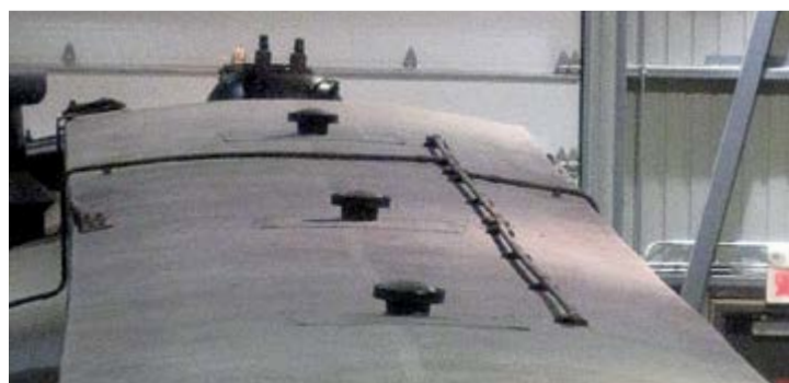
Photo 3 – Piping for gas light fixtures on roof of a wooden passenger car at Exporail. Note also that there is a mushroom vent for each light fixture. Photo by Malcolm Vant, Aug 8, 2013.
