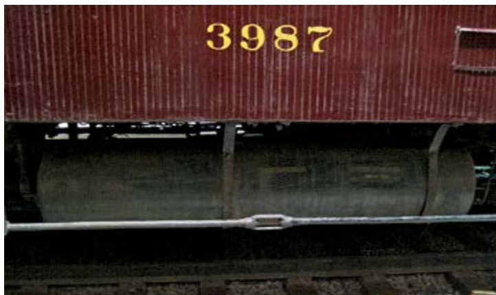
Photo 2 – Pintsch gas tank under Canadian Pacific wooden baggage car 3987, built in 1910 at Angus Shops. Photo by Malcolm Vant, at Exporail, Aug 8, 2013.
