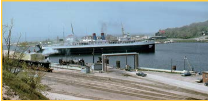
10. Above – During its time under bareboat charter to the Ann Arbor, the City of Milwaukee is entering the harbour at Frankfort, Michigan. Photos 10 and 11, taken in May 1975, show the steps in docking the ferry at the landing. The harbours used by the railroad ferries had to have a large space for the vessels to turn around before backing into the landings. Photo 10 shows it just after pulling into harbour and beginning to turn.
