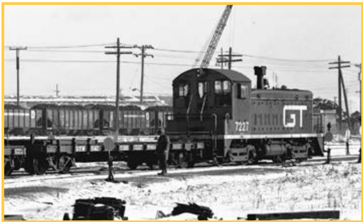
8. Below – On a bitter cold morning in February or March, 1965, the switcher and equipment at work. Note especially the idler flat cars used to reach into the ferry.
