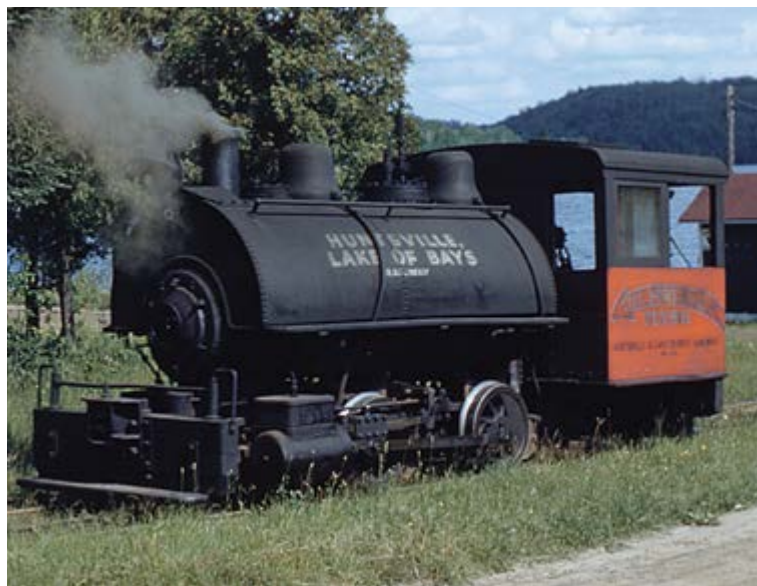
Below – The acquisition of the 17-ton MLW 0-4-0 locomotive in 1948 necessitated the railway being regauged from 44.5" to 42". W. C. Bailey, Exporail.
