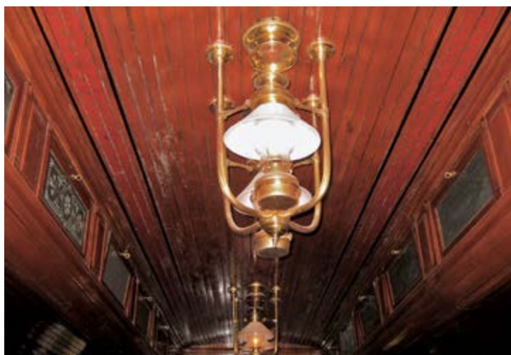
Photo 1 – Former gas light fixture, now equipped with electric bulb, in Sydney and Louisbourg car No.4, built in 1894 by Rhodes Curry, on display at Exporail, St. Constant, QC. Photo by Malcolm Vant, Sep 7, 2014.
