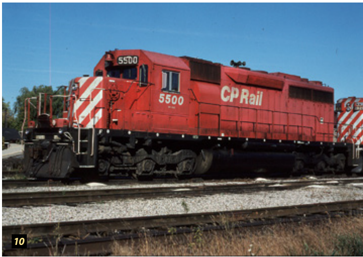
10 - CP 5500 mid-career at London, ON, on 15 October 1994. This first SD40 was delivered to CP in 1966 in maroon and grey "script" paint. Retired in 2001, she received a national Cultural Property Designation, 17 December 2003. She was then donated to the Revelstoke Railway Museum in May 2007. The trapdoor to the sand tank shows on the forward nose. Photo Glenn Courtney.
