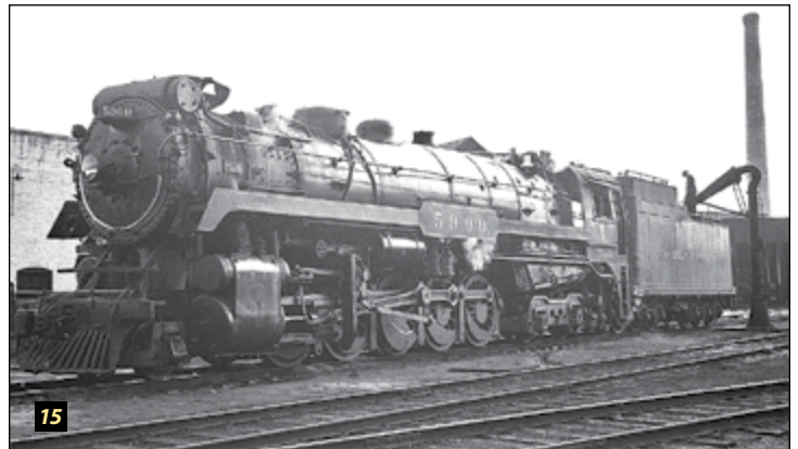
15 - Shown here in 1943, this 5900 had by then been in service in the mountains for 14 years. Revelstoke's turntable and her stall are just behind the tender, which is taking on water. The brick stack carried the exhaust of the shop's powerhouse. On the stack of the loco, its deflector has been flipped back as unneeded. When in place, it reduced the risk of knocking rock and ice off tunnel ceilings by the direct blast of exhaust. Photo courtesy of the Railroad Museum of Pennsylvania, accession No. RR75.30 (FR).
