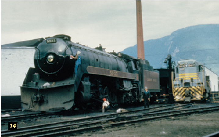
14 - This previously unpublished photo illustrates an important transition in shop power. A wiper using cotton waste soaked in coal oil is tending the jacket of class T1c No. 5933. They will carefully dispose of it in a metal container, where it will later be burned deliberately. On the ground, a machinist could be changing brake shoes while a crewman from the Geep in the background warns them of its impending movement. The year is 1959, and the smokestack in the background was the last part of the former shops to be torn down in 1988. Although rare for the time, it appears that the machinist and wiper are both women. Photo by Al Chione, Railroad Museum of Pennsylvania, accession No. RR96.36.
