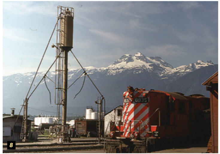
8 - The sanding facility at Revelstoke. Jack D. Thorpe photo T03-163, June 21, 1982. Photo used courtesy of the C. Robert Craig Memorial Library.
