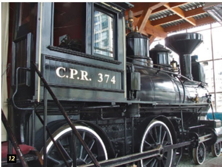
12 - Standard type 4-4-0 built May 1886 by the CPR. One of six sent to the Pacific coast immediately on completion. This engine pulled the first passenger train into Vancouver, 23 May 1887. She was modified many times over the decades until donated to the city in 1945. Now in CP's former Drake Street roundhouse, restored a second time for Expo '86. Photo TW Parkin.
