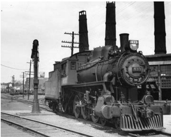
1. Diminutive 4-6-0, D4g, No. 433 beside the roundhouse at CP Ottawa West. Addy Schwalm photo.
