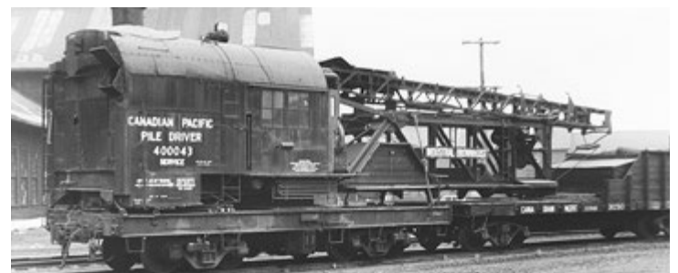
3. CP Pile Driver CP 400043, which was active on the CP roster in the 1960s, according to the CP Summary of Equipment, dated Jan 1, 1965. A Dick George photo from the Paterson-George Collection, Courtesy of Dave Stremes.
